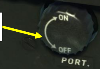
Portside (Left) Flood Lights Control Knob
