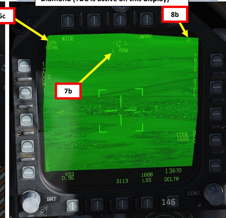
TDC (Throttle Designator Controller) Focus Diamond (TDC is active on this display)
