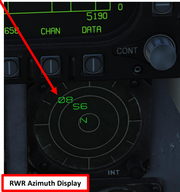
OFFSET can be seen as a RWR de-clutter function
