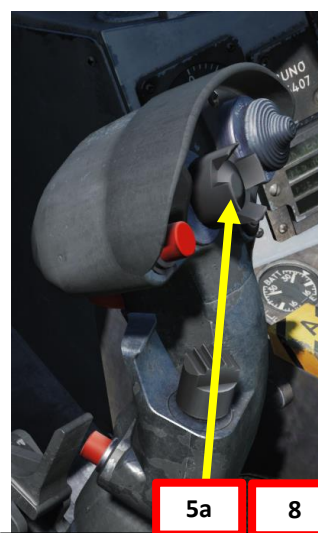
Sensor Control Switch AFT/FWD/LEFT/RIGHT/DEPRESS
