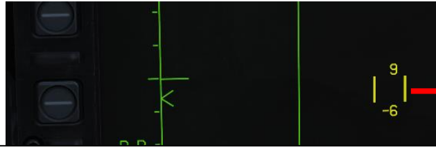
TDC (Throttle Designator Controller) Acquisition Cursor Upper number: Upper altitude covered by radar (9000 ft) Lower number: Lower altitude covered by radar (-6000 ft)
